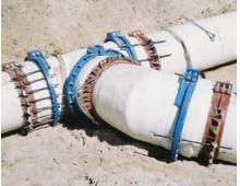
The PV-LOK™ Series PVPF (left) is used to restrain PVC Pipe at gasketed PVC fittings. Restraining rods are included in the kit to connect the PV-LOK restrainer, to the included two piece beveled back up ring that seats behind the bell of the PVC fitting.
