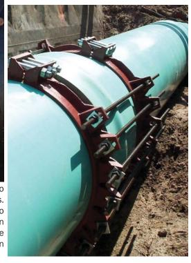
The PV-LOK™ Series PVP (right) is used to restrain PVC Pipe at bell and spigot joints. Restraining rods are included in the kit to connect the two PV-LOK restrainers, one on each side of the bell joint. In sizes 4-16″ the Series PVP can also be used on ductile iron pipe bell joints.
